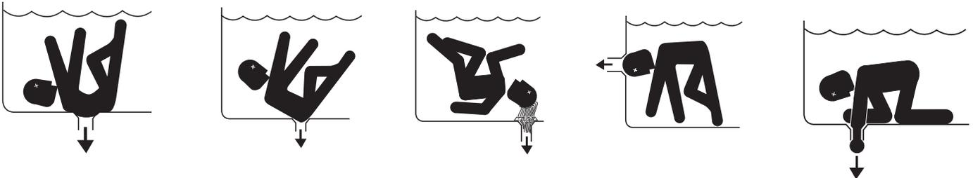
Pool and spa pumps produce high levels of suction, which can pose extreme danger if a person comes in close proximity to an open pool or spa drain or if a drain cover is loose, cracked, broken or missing. Pool and spa pumps move large volumes of water, which can pose extreme danger if a person's hair comes in close proximity to a drain that is not the proper size for the pump or pumps.
