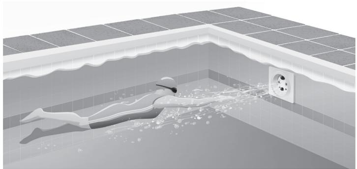
*NOTE: Under certain conditions it is possible that the current “drifts off” to the left or the right from the middle due to water bouncing off the back wall. In the event that it interferes with your swimming action, turn the unit OFF for a few minutes and restart.*
