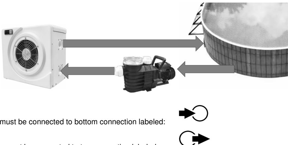
Inlet water tube must be connected to bottom connection labeled:
